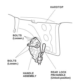
• Open the front lock handles. With the help of an assistant, gently set the front of the hardtop on the windshield frame, and align the front lock handles with the front strikers. At the rear of the hardtop, fit the roof lock pins through the holes in the body side catchers.
