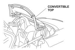
2. Locate the link stopper. Apply weatherstrip adhesive to the inside of the rubber spacer and attach it over the link stopper. Repeat on the other side; then lower the convertible top completely.
