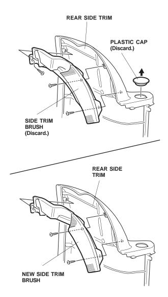
12. Get the right rear side trim, removed in step 5. Repeat step 11 to install the new right side trim brush to the right rear side trim.
