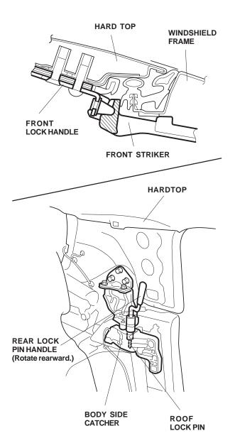
Lock the front of the hardtop into position with the front lock handles, and lock the rear of the hardtop by rotating the rear lock pin handles rearward into the *lock* position.
